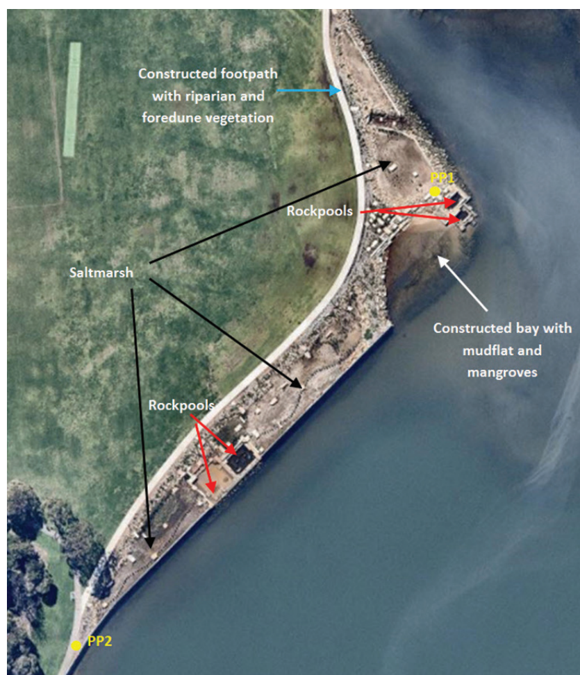
Figure 3. Aerial of completed seawall identifying key features. (PP - Photo points).
